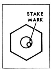
In order to remove a diode from the **end frame**, drill a 3/16" hole 1/8" deep into the stake mark to relieve the pressure between the threads. This operation will avoid damage to the end frame threads that otherwise would occur during removal.
