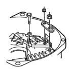
4. Remove regulator stud connector from inside slip ring end housing by removing regulator stud nut and inside output (BAT) terminal nut. Note that output (BAT) terminal may fall out when nut is removed. Also remove insulated regulator attaching screw.
